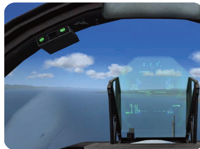
Fig. 12 READY, LEFT and RIGHT Advisory lights.
