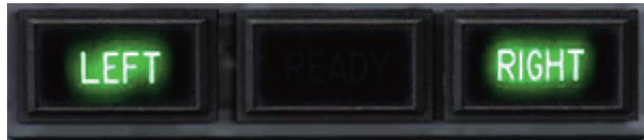
Fig. 14 LEFT and RIGHT Air refueling lights
