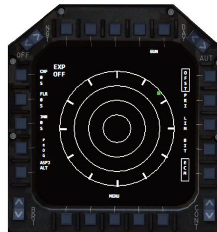
Fig. 90 ECM Display. RWR ON, Expendables OFF.
