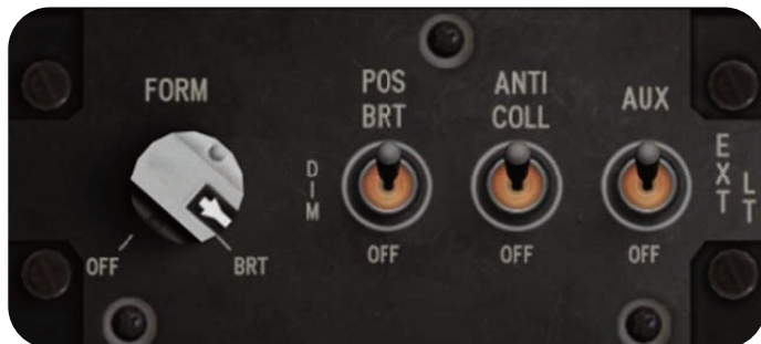
Fig. 17 Exterior Lights Panel
