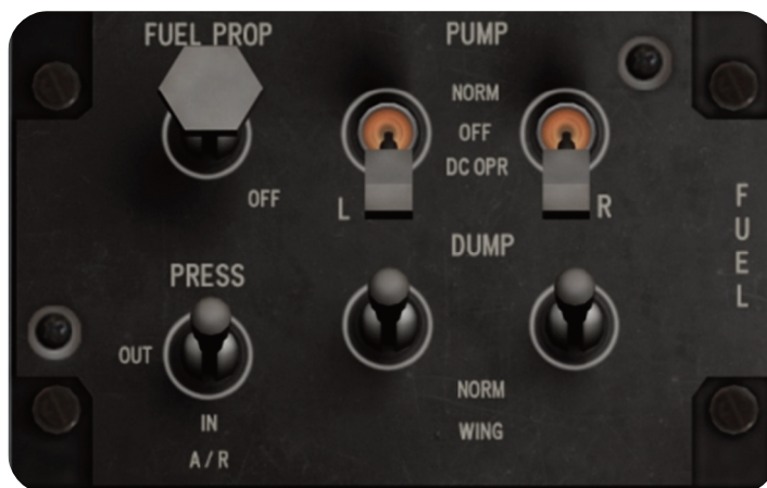
Fig. 11 Fuel Control Panel
